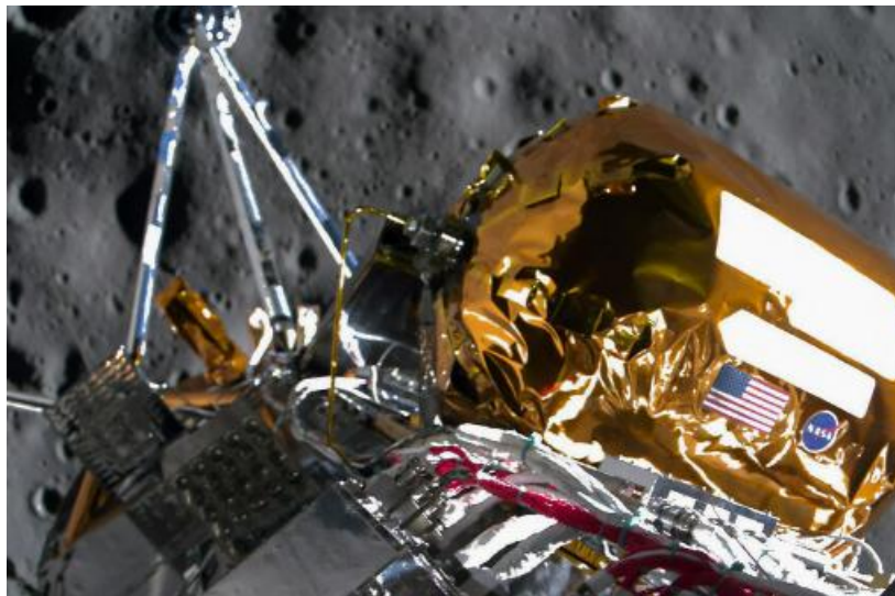
Independence payload mounted on the Odysseus lander on the lunar surface during the successful 2024 IM-1 mission.
